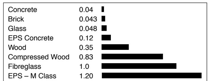
Figure 8: Typical R-values, various insulating materials 50mm thick
