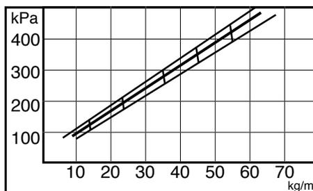
Figure 4: Shear strength v density at 23°C
