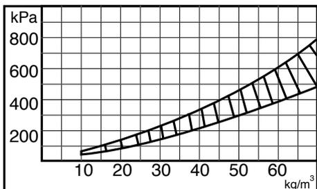
Figure 1: Compressive stress at 10% deformation v density
